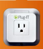
The Plug-IT 110 provides on/off control for 110 volt 15 Amp applications. Each Plug-IT contains a microprocessor which communicates with the JACE control software using your WiFi network. Each Plug-IT is individually named and remembers complex on/off schedules that can be changed remotely with a click of the mouse.
